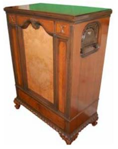
Kolster K-45 Console Radio – An 11-tube radio that covered the AM band and was AC powered, this handsome set was made in 1928 and originally had a remote control. The output was two #50 tubes. It originally cost \$500 when introduced. Gregory Jones, San Leandro, CA
