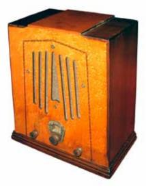
**National SW-3 Receiver** - Made in the early 1930s, this was a simple regenerative receiver. It used three tubes: 58, 58, 56. Originally came with three sets of coils for different bands. Arnold Corwin, Memphis,TN
